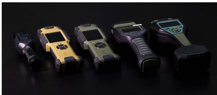
爆炸物与毒品便携式检测装置 Portable detection devices for explosives and narcotics
